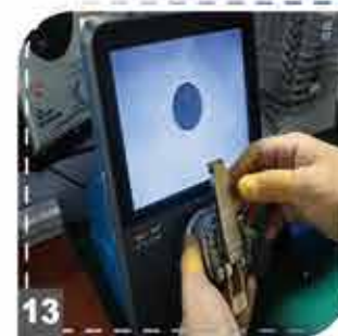
13 Check and clean module optical end face
